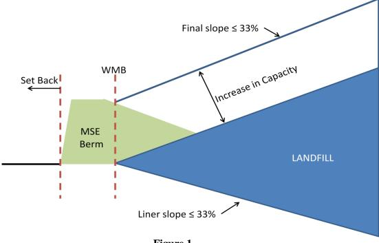
**Figure 1.**MSE Berm addition without changing the WMB
